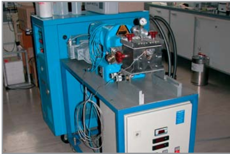
Sigma blade compounder for developing new feedstocks Batch size 750 cm 3 , temperature up to 280 °C, wear-resistant lining.
