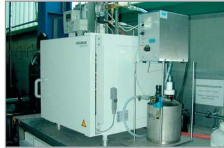
Catalytic debinding furnace: Working temperature 120 °C, HNO 3 catalyst in N 2 atmosphere for CATAMOLD® feedstocks (BASF).
