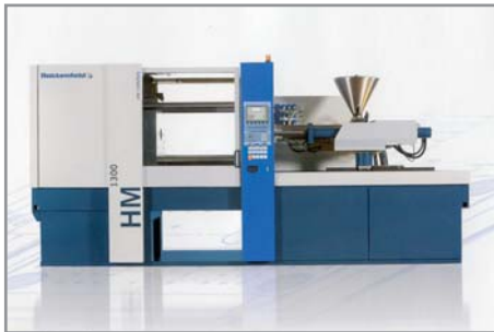
Injection molding machines: Clamp force 40 and 50 tonnes, adapted for PIM materials.
