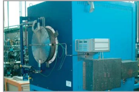
Thermal debinding furnace: Temperature up to 1000 °C (vacuum, reducing, oxidizing, and inert atmospheres), muffle size 30 liters, binder trap, burn-off stack.
